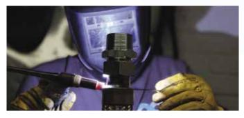
In addition all welds used in the production of metallic braided hose assemblies and pipework fabrication are also covered by TUV individual WPS's (weld procedure specification) and WPQR's (weld procedure qualification records). Once again please consult our team for further details.
